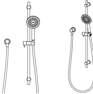
1. Supplied with the Flow Regulator prefitted - attach to the hose and place in slider
