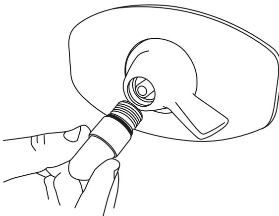
2. Screw the elbow end with the black 'o-ring' into the wallset. The plastic flange provided will not be needed for this conversion.
