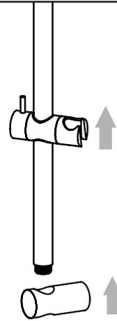
6. Fit slider first onto the rail and lock it halfway up. Then fit bottom mounting bracket onto the rail.
