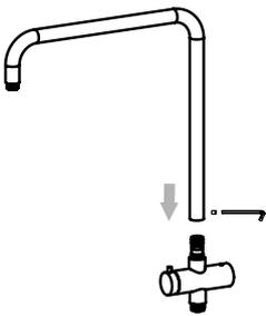
4. Fit overhead shower arm onto diverter valve and secure grub screw on shower arm into the white bushing using the 2.5mm allen key.
