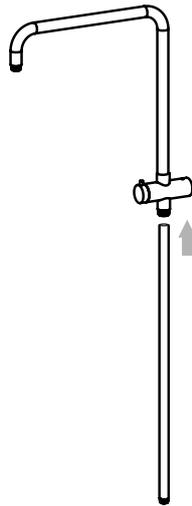
5. Screw bottom rail section onto diverter valve.
