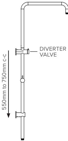
Mark down vertical between 550mm and 750mm from centre of water outlet.
