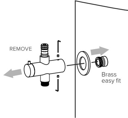
2. Loosen grub screws on body of diverter valve using a 2.5mm allen key. Withdraw the brass easy fit. Screw easy fit onto water outlet till it is flush against the wall face; slide chrome flange over the easy fit.
