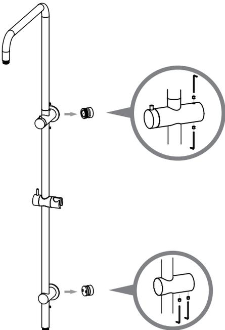
7. Fit the entire assembly onto wall by tightening the grub screws on the bottom and top mounting bracket using the 2.5mm allen key.
