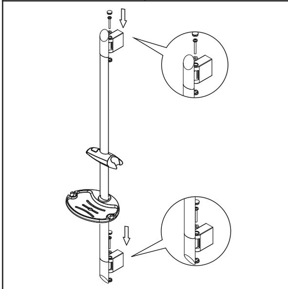
5. Secure brackets with bracket screws and caps provided.
