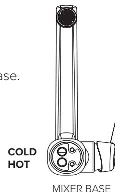
**Maximum bend for flexible hose is 35mm radius. The nipples on the hoses must be connected to fittings which have machined end faces, not "sawn off" threaded tube.**
