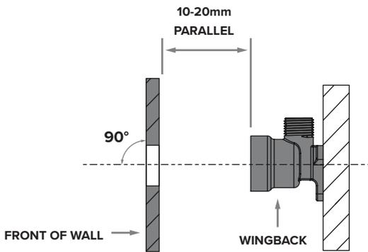
1. Ensure the wingback when fitted is parallel and square to the finished wall lining as shown
