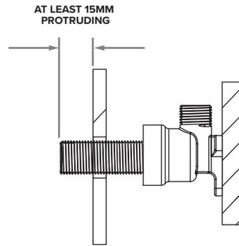
2. Cut and fit 1/2" BSP with at least 15mm protruding from the finished wall. Use seal tape when threading into wingback.
