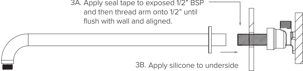
3B. Apply silicone to underside of flange and fit until contact on wall.
